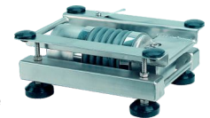
Waterproof platform scales feature bellow-type mechanical design aiming to protect strain gauge transducer against ambient conditions effect
