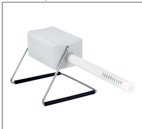
**The THB 3 module** is a measuring device cooperating with the newest series of automatic mass comparators and manual comparators but also with 3Y series laboratory scales, a PC computer and the THB-R recorder. THB 3 module serves for measuring the three following parameters directly from the measuring position, the temperature parameter, the humidity parameter and the atmospheric pressure parameter.
