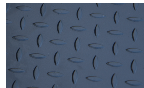
The upper part of the weighing pan is a tear plate surface
